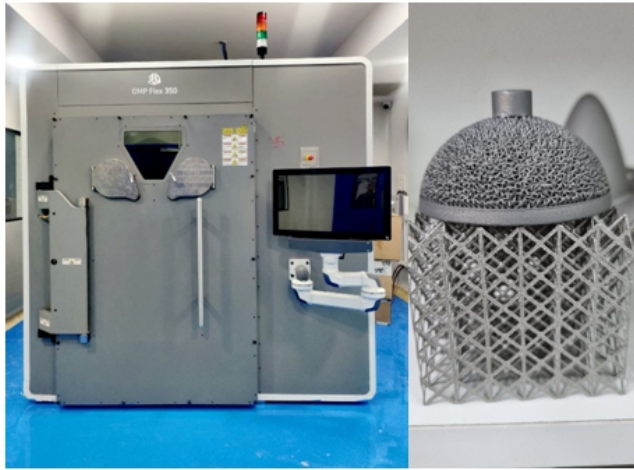
3D Printing Machine and Lattice structure / Trabeculae cup
